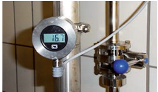
Tube-mounted sensor GTL 737 with LC display
