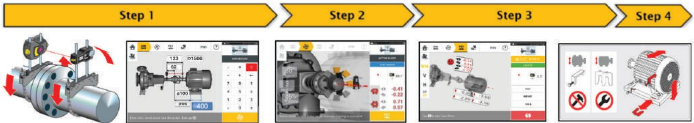
1. Mount the brackets on either side of the coupling. The reflector should be mounted onto the machine to be moved (motor) while the sensor unit is mounted on the stationary (driven) component.
