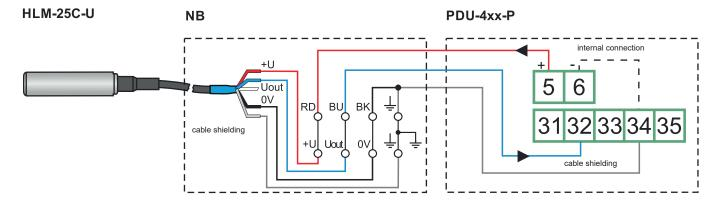
Connection diagram - level meter with voltage output to PDU unit, using internal power source
