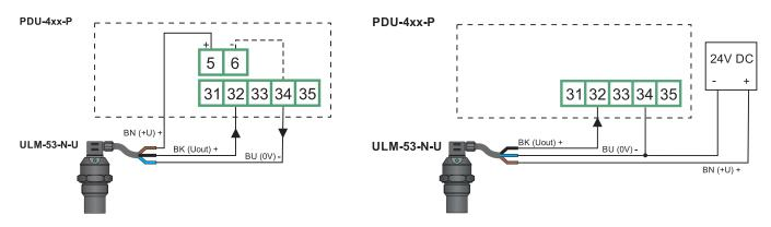
Connection diagram - level meter with voltage output to PDU unit, using internal power source
