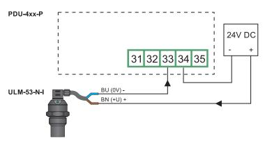
Connection diagram - level meter with current output to PDU unit, using external power source
