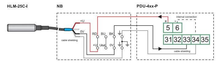
Connection diagram - level meter with current output to PDU unit, using internal power source
