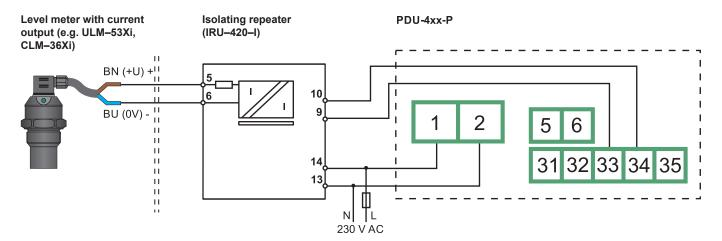
Connection of the unit to the level meters with current output located in explosive areas
