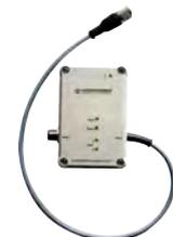
If required, all parameters can be set at any time on all intelligent sensors, using the ECI-1 device configurator.
