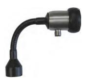
A gooseneck between the electronics head and the primary sensor provides freedom in the orientation of the sensor. This option simultaneously provides thermal decoupling between the two units. The length of the gooseneck is 140 mm.
