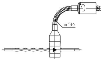
A gooseneck (optional) between the electronics head and the primary sensor provides freedom in the orientation of the sensor.
