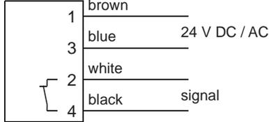
The switching outputs are self-configuring, depending on whether they are connected as PNP or NPN switches.
