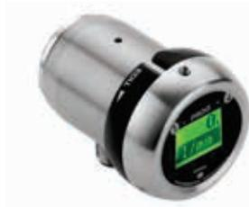
This OMNI electronic option should be used where temperatures change quickly, or for external installations (the device is filled with oil, and thus prevents condensate formation in the electronics housing, even under adverse circumstances)
