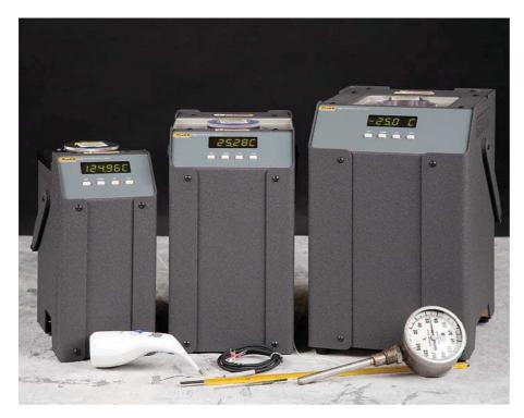
You may have noticed we haven't touted our CFC-free refrigeration. Yes, cold Micro-Baths are CFC-free, and also compressor-free. That's right—no heavy, noisy compressor to lug around. We achieve our temperature range and stability with only one moving part. This means more durability and less weight.
