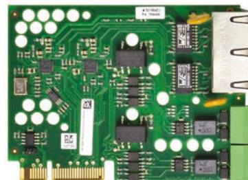
The communications card is equipped with 2 Ethernet ports (IEEE 802.3) and 2 RS485 interfaces.
