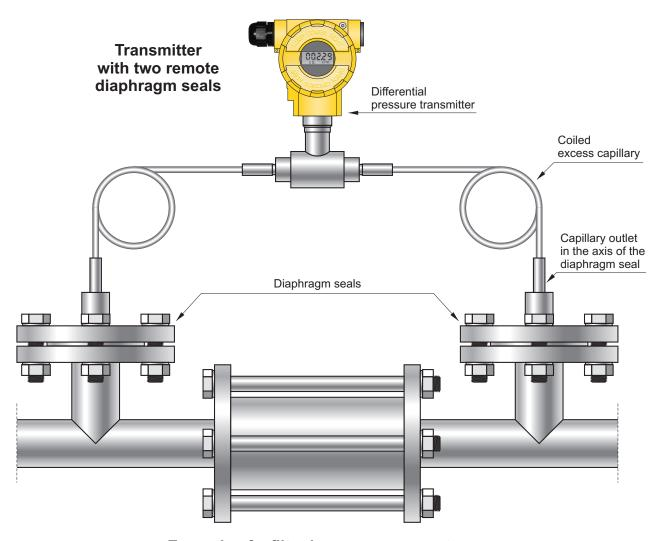
Example of a filter loss measurement
