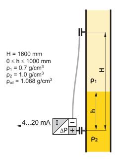
To determine the start of the measurement range, calculate the pressure difference at the transmitter when the tank is filled with the lighter liquid only:
