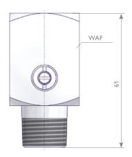
Gauge Snubber Type made from 32 mm square barstock material.
