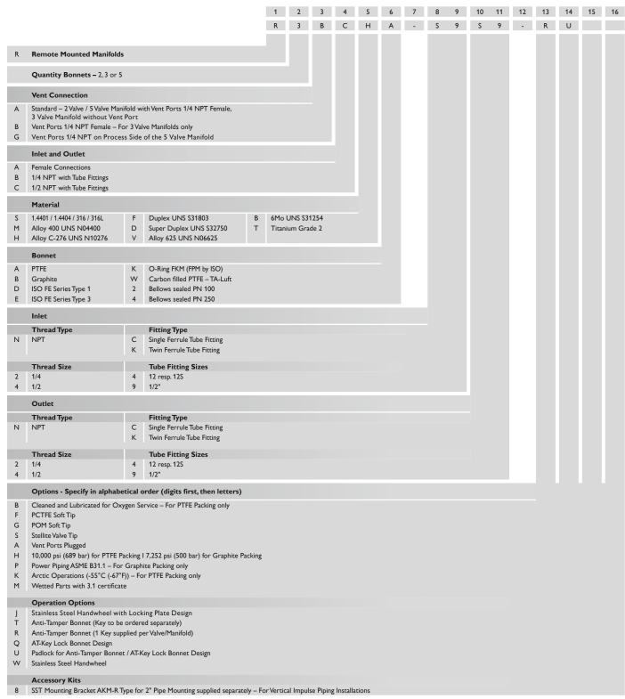
Wetted Parts according to a.m. material list are supplied according to NACE MR0175/MR0103 and ISO 15156 (latest issue) - except Titanium Grade 2. Note: Not every configuration which can be created in the ordering information is feasible / available.
