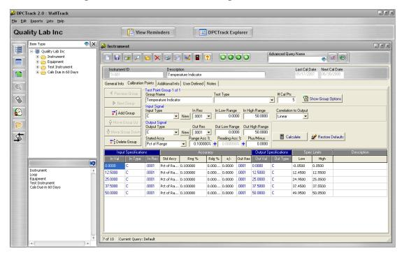
Fluke 750SW DPC/TRACK 2 software includes aninstrumentation data-base that makes it easy to manage your instrumentation, create and schedule tests, load and unload the 753 or 754, print a variety of standard reports, and manage calibration data.
