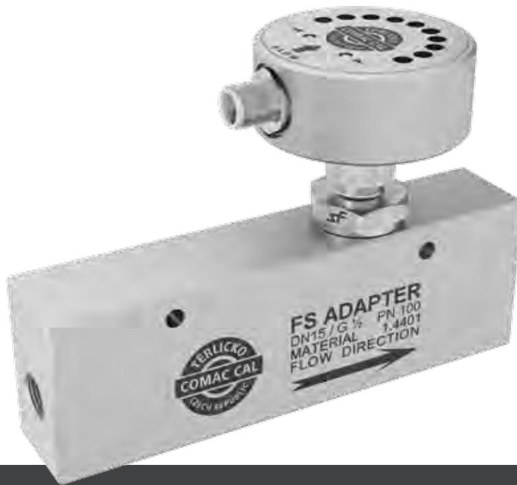
In case when it is necessary to monitor the media flow in the pipe with a smaller DN than DN 25 (or the flow velocity is below the sensor range at the pipe diameter given), it is possible to use an adapter block with a corresponding flow velocity and ensure correct operation and keep the installation conditions in this way.
