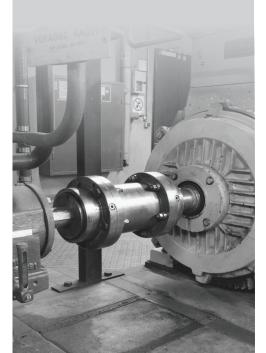
It's a known fact—all rotating machinery is susceptible to misalignment. Machines that are well aligned at the commissioning stage and regularly maintained will have reduced wear in couplings, bearings, and seals, all of which means reduced plant operating and maintenance costs.
