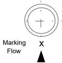
Avoid bubbles or deposits on the sensor. It is therefore best to install at the side. For T-pieces or welded-on nozzles, see Accessories.
