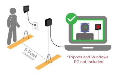
Seek Scan<sup>™</sup> is a simple, low-cost, thermal imaging system designed to automate body temperature screening using skin temperature as a proxy. With ±0.3°C (±0.5°F) accuracy and the inclusion of a reference heat source, Seek Scan delivers the same performance as an infrared temporal thermometer – but with a safe social distance.
