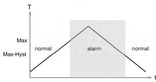
While in the normal state the switching outputs are at the level of the supply voltage; in the alarm state they are at 0 V, so that a wire break would also display as an alarm state at the signal receiver.
