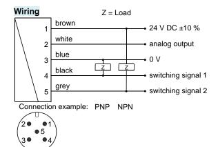
Before the electrical installation, it must be ensured that the supply voltage corresponds to the data sheet.
