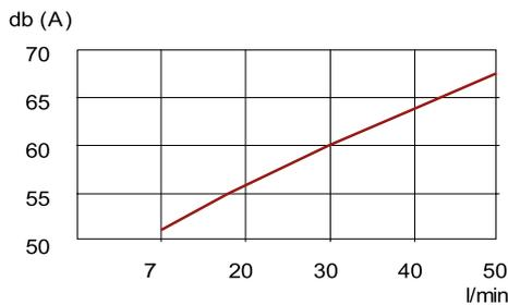
The noise level always remains below the curve with the specified flow value. Test viscosity was 22 mm²/s. With a higher viscosity the noise level is lower.
