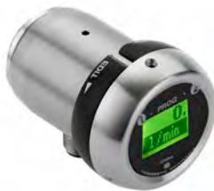
This OMNI electronic option should be used where temperatures change quickly, or for external installations (the device is filled with oil, and thus prevents condensate formation in the electronics housing, even under adverse circumstances)
