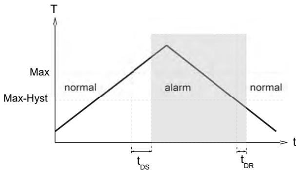
be applied to switching back to the normal state. In the normal state the integrated LED is on, in the alarm state it is off, and this corresponds to its status when there is no supply voltage.
