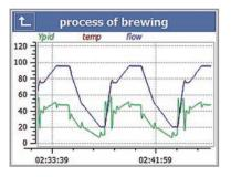
The trend representation is independent of the logger function, and so various process signals can be displayed and recorded. The library also provides an alarm block. this block can be used to display alarm lists in plain text on the device. The alarms can be acknowledged on the device and even used for further processing within the application.
