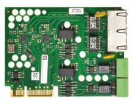
The communications card is equipped with 2 Ethernet ports (IEEE 802.3) and 2 RS485 interfaces. Ethernet
