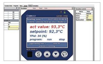
An essential point is the PC simulation of the complete application. The entire application can be tested on a PC independently of the actual process. For this purpose, the CAT software has a simulation environment for the MSR 9696H and for connected I/O assemblies. With this environment, the user is capable of testing the entire application, including operation on the PC, without endangering the real process. Simply test the application at a desk without risk.
