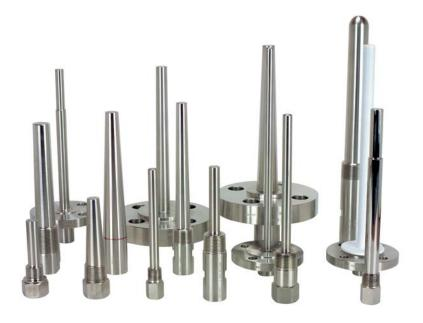
Thermowells are used to protect bulbs from the effects of corrosion and pressure, from the process fluid flow velocity and to allow the thermometer to be interchanged, recalibrated, or replaced, without affecting the process.
