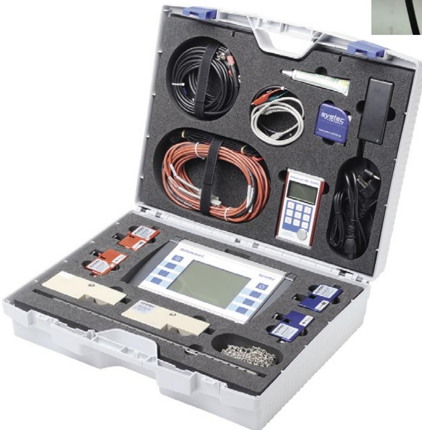
The mobile deltaxwaveC-P measuring device comes in a robust practical carrying case complete with flow transmitter, ultrasonic transducers, installation material, signal cable and coupling grease, SD memory card and power supply.
