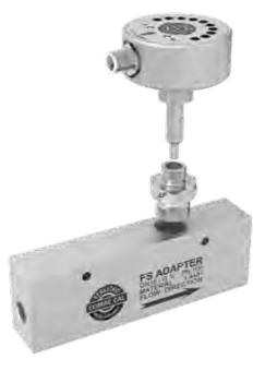
In case when it is necessary to monitor the media flow in the pipe with a smaller DN than DN 25 (or the flow velocity is below the sensor range at the pipe diameter given), it is possible to use an adapter block with a corresponding flow velocity and ensure correct operation and keep the installation conditions in this way.
