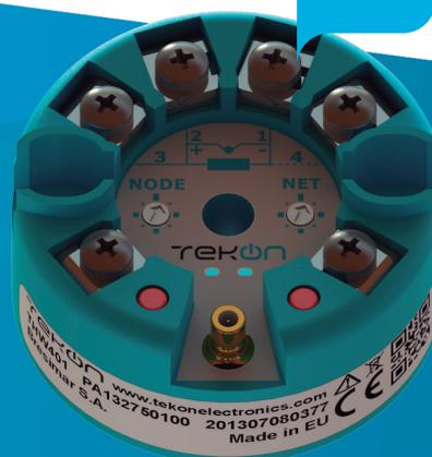
The Universal Wireless Temperature Transmitter THW401 is specifically designed to meet the most rigorous requirements of operation in the industrial process environments. Due to its reduced dimensions, it may be installed in the DIN Form B sensor connection head, in place of the traditional terminal blocks or current loop temperature transmitter.
