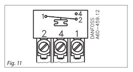
KPS thermostats are fitted with a Pg 13.5 screwed cable entry suitable for cables from 5 – 14 mm. Contact function is shown in fig. 11
