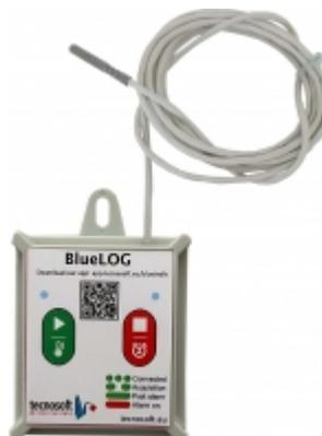
By connecting a Bluetooth thermal printer you can print the data to be attached to the documents upon delivery. The **batteries are replaceable by the user** and the **Accredia traceable calibration certificate** can be requested separately.
