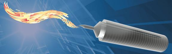
PressureDisk is a temperature and pressure data logger from -40°C to 140°C (calibration from 25°C to 140°C) and from 0 to 5 bar with 20 mm length external probe, managed with Windows software and USB interface (DiskInterface HS, Multibay). **Battery is user replaceable** and the data logger is **provided with an Accredia (NIST equivalent) traceable certificate** on different points.
