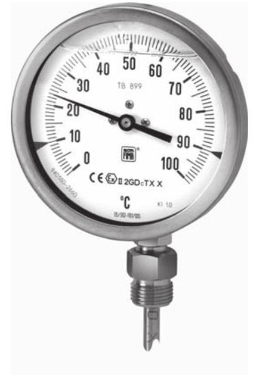
These instruments are designed for explosive atmospheres in food, processing, pharmaceutical, petrochemical industries and conventional and nuclear power plants. They are in conformity with the essential Health and Safety Requirements laid down in European Directive 2014/34/UE for Group II, Category 2G or 2GD equipment in the T1...T6 temperature classes. They are NOT suitable for ZONES 0 and 20.
