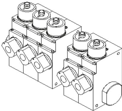
The limit switch can be used to monitor minima or maxima. With a minimum-switch, falling below the limit value causes a switchover to the alarm state. Return to the normal state occurs when the limit value plus the set hysteresis is once more exceeded.
