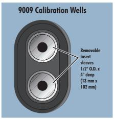
Each block contains two wells, which accept removable inserts. A 1/4" and a 3/16" insert are included for each block. Additional sizes (including custom sizes) are available.
