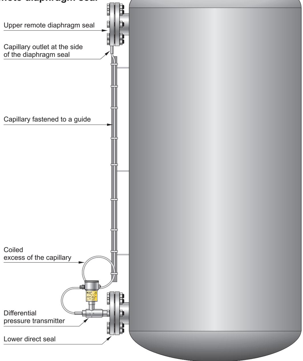
**Example of measurement of the level in a pressure tank**
