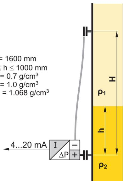
To determine the start of the measurement range, calculate the pressure difference at the transmitter when the tank is filled with the lighter liquid only:
