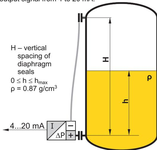
1. Install the transmitter in its working position on an empty tank.
