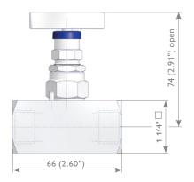
Hand Valve with Integral Tube Fittings HATT Type
