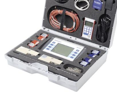
The mobile deltawaveC-P measuring device comes in a robust practical carrying case complete with flow transmitter, ultrasonic transducers, installation material, signal cable and coupling grease, SD memory card and power supply.
