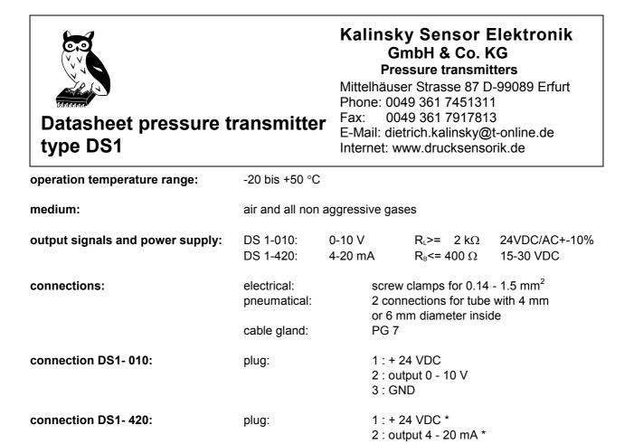
\* Because of a additional special circuitry the transmitter can't be damaged due to a wrong connection. *That means*: both wires can be changed. Between 2 and GND of the power supply must be
