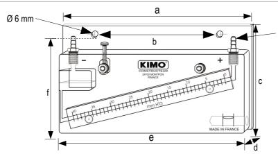
Cylindrical 1/8 gas connector  $\emptyset$  6.2 mm ribbing
