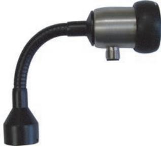
A gooseneck between the electronics head and the primary sensor provides freedom in the orientation of the sensor. This option simultaneously provides thermal decoupling between the two units. The length of the gooseneck is 140 mm.
